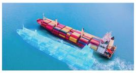
shipbuilders to test and optimize systems before physical implementation, reducing the time and cost associated with sea trials. Also, by monitoring the health of the machinery in real time, digital twins can predict when a component is likely to fail and alert the crew to perform the right maintenance before a breakdown occurs. The upper example highlights the proactive nature of the digital twin technology through predictive maintenance.
